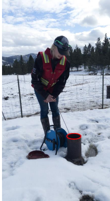
Figure 7: Wells that stick up above the ground surface (stick-up height) are measured from the top of the casing (red circle).
