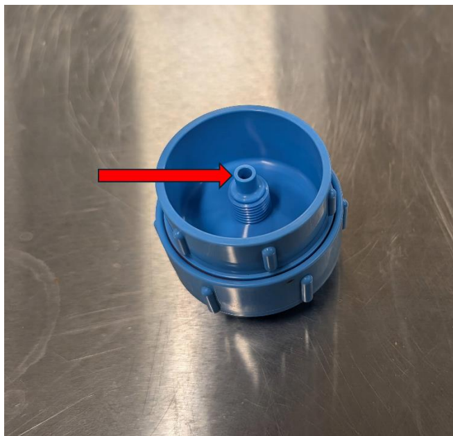
Figure 5: The port on the bottom of the filter holder accepts a standard 60mL syringe tip. Be careful to avoid damaging the syringe and filter holder when inserting the syringe.
