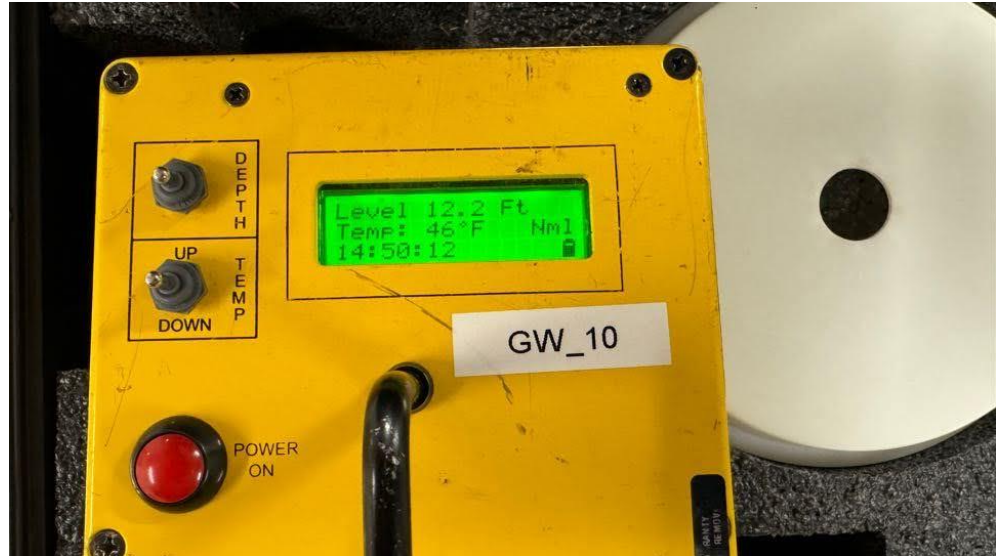
Figure 9: Control interface for the Sonic. The RED Power ON button also triggers a measurement from the instrument.
