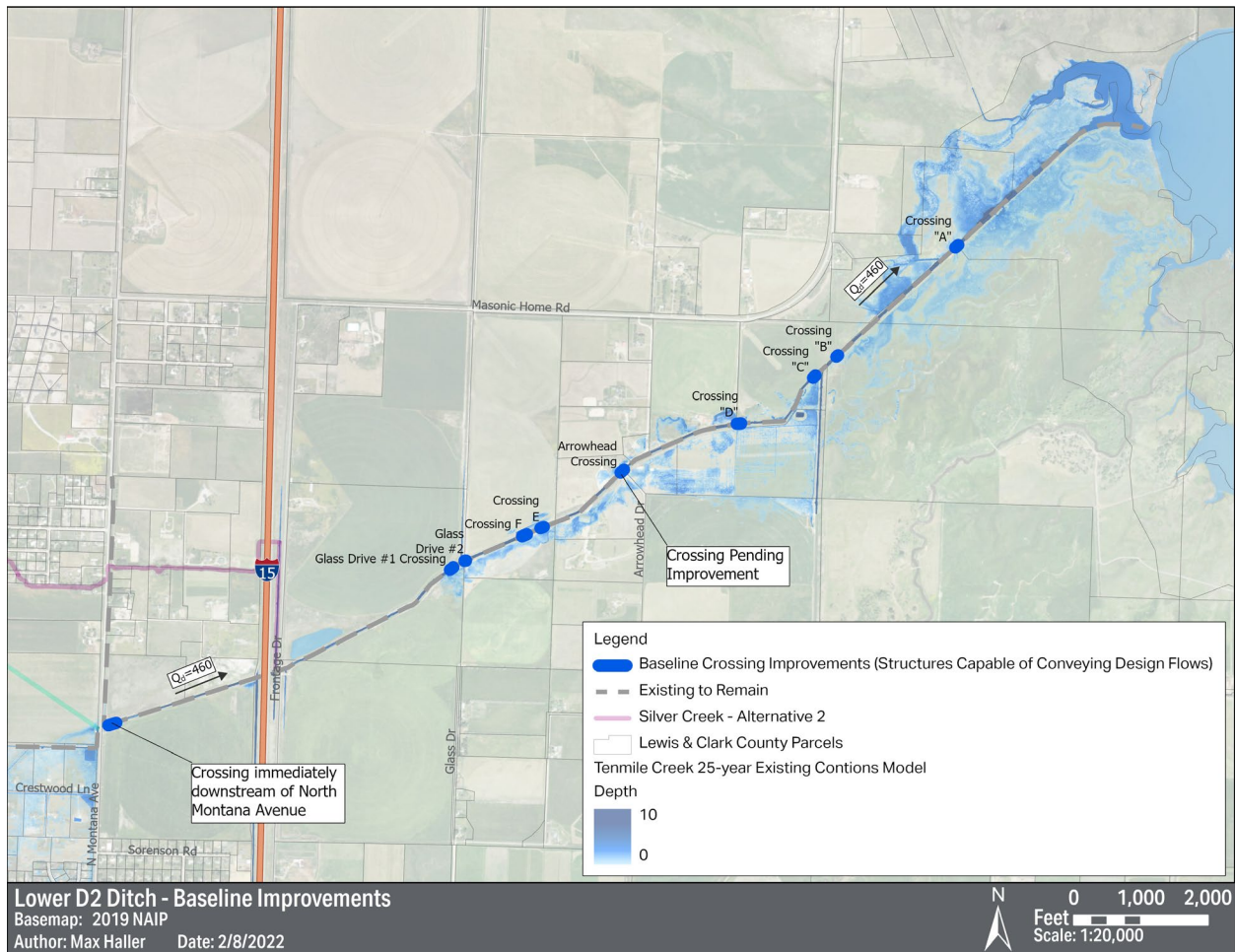
Figure 3-1. Baseline Improvements for the D2 Ditch with the Tenmile Creek Existing Conditions 25-year model results.
